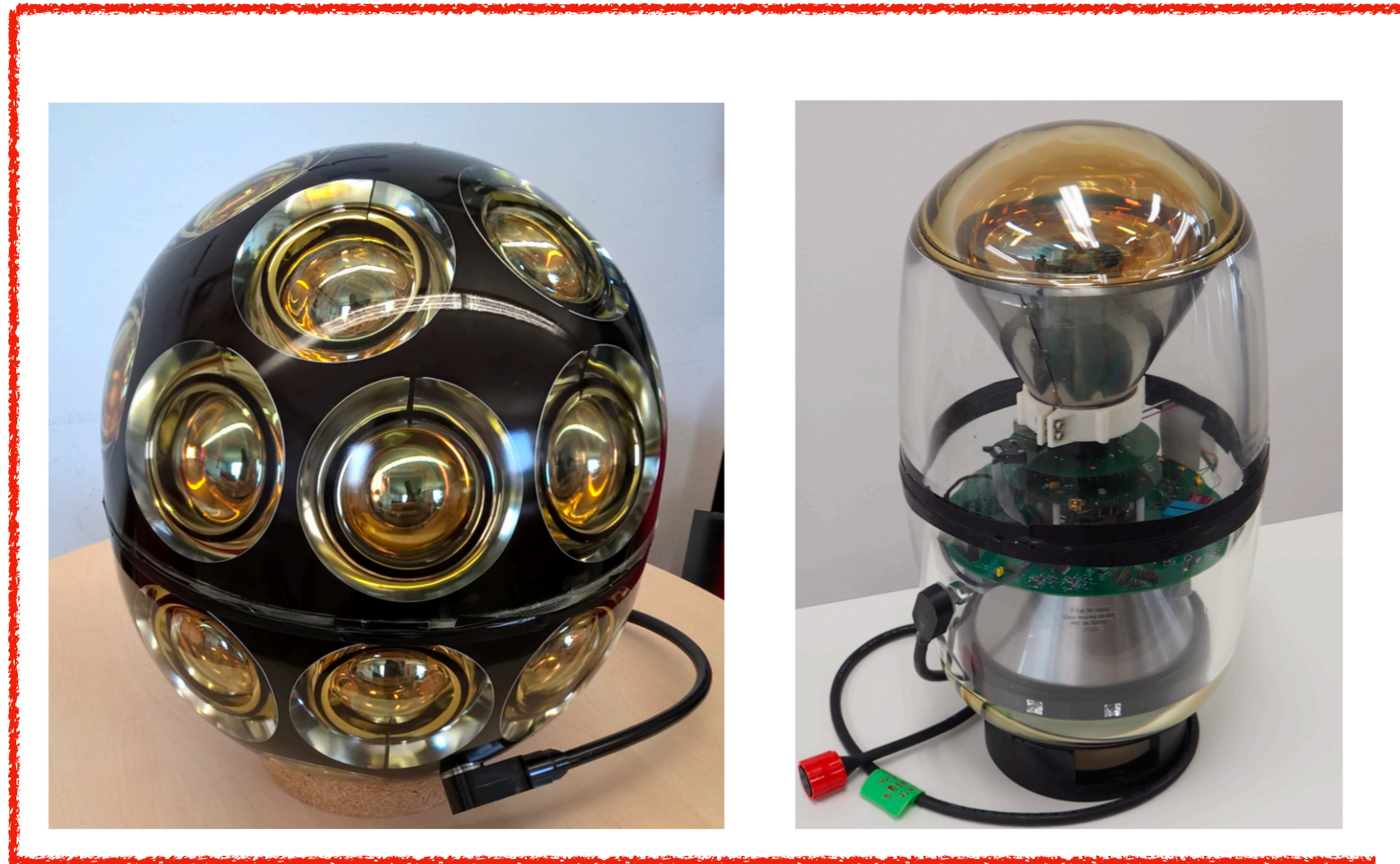
Directional information 24 x 3 inch PMT Diameter 36 cm
